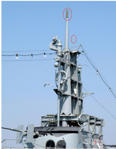
Target & attack periscopes
