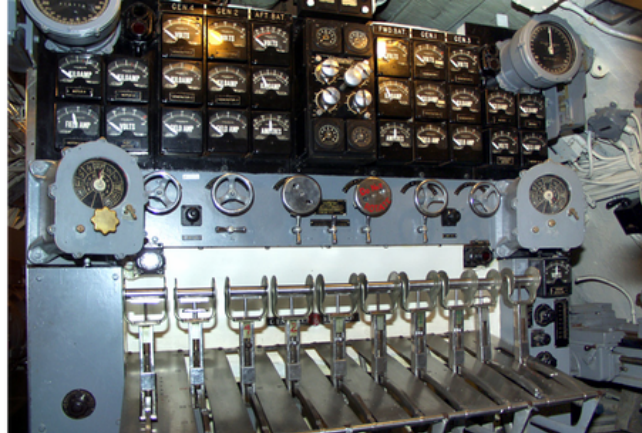
4 million watts can pass through this cage This panel controls the ship's propulsion when underway
