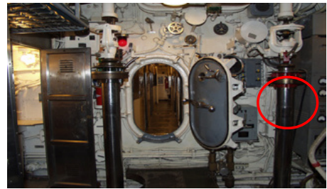
Active sonar heads on either side of hatch to “Officers country”
